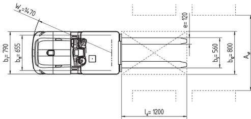
Single lift mast 1500 without auxiliary lift
